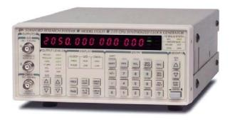
The CG635 synthesized-clock generator produces extremely clean, low-jitter clock signals over a frequency range of 0.001 Hz to 2.05 GHz. The cost is a fraction of that of RF synthesizers, which, until now, have been the only type of instrument suitable for producing many of the clock signals the new generator produces.
